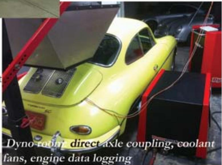
*Dyno room, direct axle coupling, coolant fans, engine data logging*
