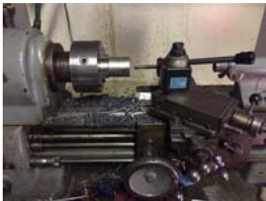
Boring out the height adapters on the lathe
