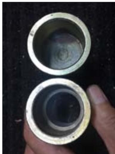
Height adapters before and after boring for screw clearance
