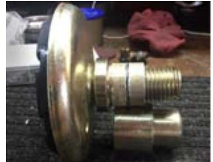
Threaded stem could not screw all the way down.
